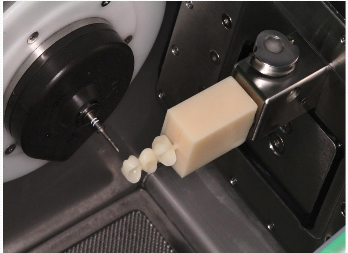
Freshly milled restoration.
